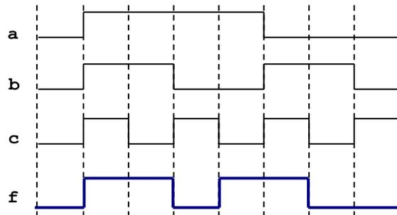
b) Complete the timing diagram of the logic circuit whose VHDL description is shown below: (5 pts)
